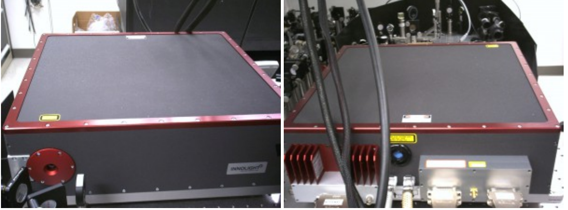
Figure 3.3: Front (left) and rear (right) of the MOPA, the master laser used in the experiment. Black desiccant cartridge visible at center of rear; center indicator is dark blue when the cartridge is fresh, exchange cartridge when it turns light purple.
